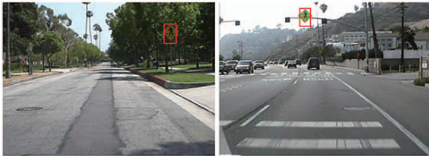
Fig. 3 Illustration of similar false positives obtained from in-vehicle camera images having different appearances
