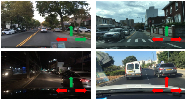
FIGURE 1. Typical scenes in the BDD-3AA dataset. As shown in the upper left image, there are double yellow solid lines on the left, thus the steering left action is not available; there are vacant spaces in the front and right, thus the acceleration and steering right actions are available. The green arrow denotes the corresponding action is available, the red arrow denotes not available.
