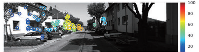
(b) Depth at image feature points (Color: distance [m])
