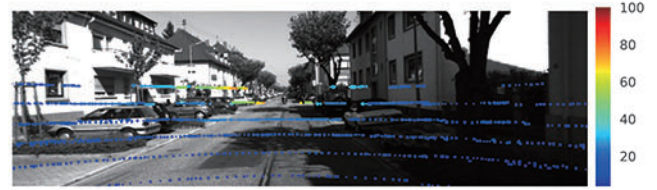
(a) LiDAR points overlaid on an image (Color: distance [m])
